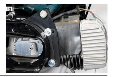
Place the O-ring in the hollow under the valve support and tighten with 4 M5x10 countersunk screws. Mount the reed valve, the gasket and the manifold with M5x20 screws (photo 14).
