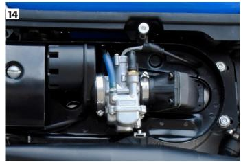
Mount the carburetor and the filter. Install the transmission and adjust the belt. Complete with the tightening of the engine screws on the frame including the M6x35 screw with spacer (photo 15).
