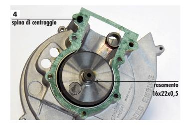
Close the crankcase by inserting the M6x40 TE screws on the flywheel side at 12Nm or 1.2Kgm with M6 nuts and 6x13x1,5 washers; cut the gasket (photo 5).
